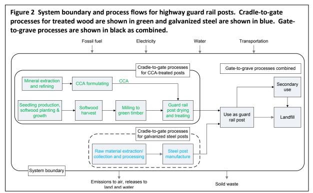
The system boundaries include all the production steps from extraction of raw materials from the earth (cradle) through to final disposition after service life (grave). Figure 2 illustrates the system boundaries and process flow for both wood and non-wood highway guard rail posts assessed in this study.
